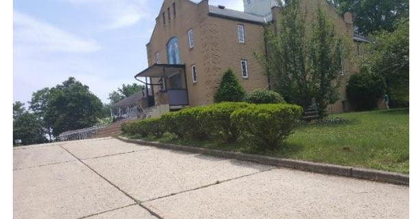
Two rows of parking spaces can be converted into pervious pavement to infiltrate runoff. The church also has two downspouts in the back which can be disconnected and directed into a rain garden to capture, treat and infiltrate runoff. A preliminary soil assessment suggests that the soils have suitable drainage characteristics for green infrastructure.
