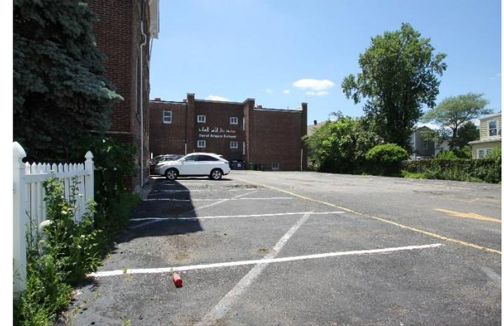
The parking lot is in fair condition and is a good candidate for pervious pavement. Additionally, downspouts in the front of the building can be directed into planter boxes and rain gardens to capture, treat, and infiltrate runoff. A preliminary soil assessment suggests that the soils have suitable drainage characteristics for green infrastructure.
